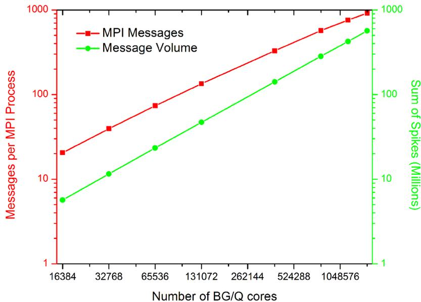
(b) Average counts of MPI messages per Compass MPI process and spikes received across all processes, per simulated one-millisecond TrueNorth tick. We show the counts for the weak-scaling experiments only.
