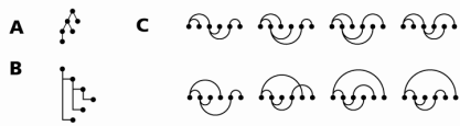
Figure 12. Tree Diagram (A) and Tree Table (B) oversimplify the conversational structure of a thread. The 8 Thread Arcs (C) reveal different ways the conversation may have evolved.
