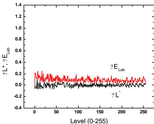
Figure 6. Calculated Lab  $\Delta E$  and  $\Delta L^*$  errors for 10-bit conversion from D65,  $\gamma=2.2$  to D50,  $\gamma=1.8$ .
