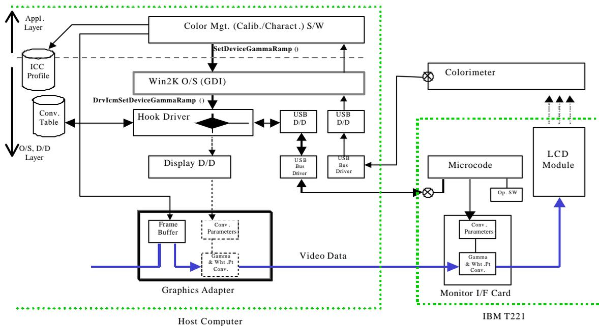
Figure 1. Block diagram of color management function utilizing monitor color LUT.
