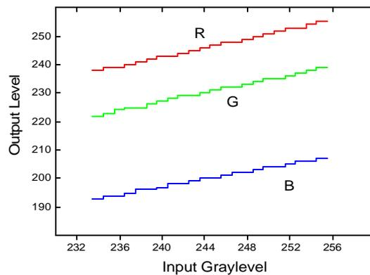
Figure 4. Degeneracy errors introduced at high end.
