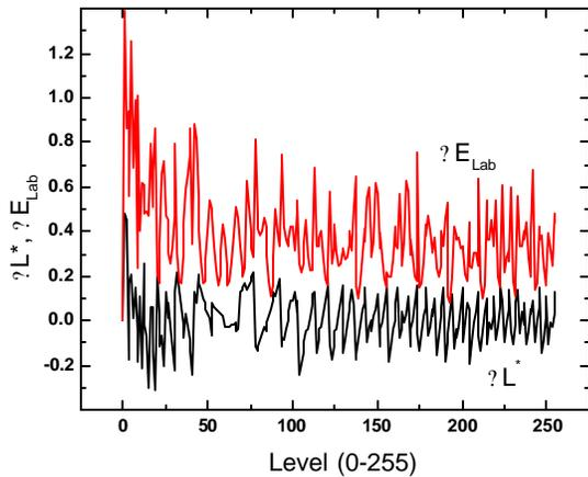
Figure 5. Calculated Lab  $\Delta E$  and  $\Delta L^*$  errors for 8-bit conversion from D65,  $\gamma=2.2$  to D50,  $\gamma=1.8$ .
