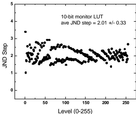
Figure 8. DICOM results for 10-bit calibration.
