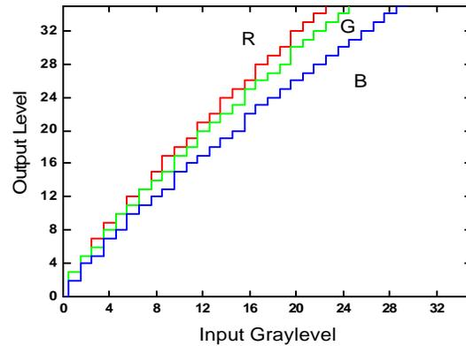
Figure 3. Quantization errors introduced at low end.
