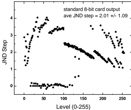
Figure 7. DICOM results for 8-bit calibration.
