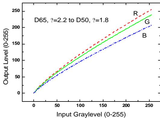
Figure 2. Table for changing D65 whitepoint and 2.2 gamma to D50 and 1.8 using 8-bit to 8-bit conversion.
